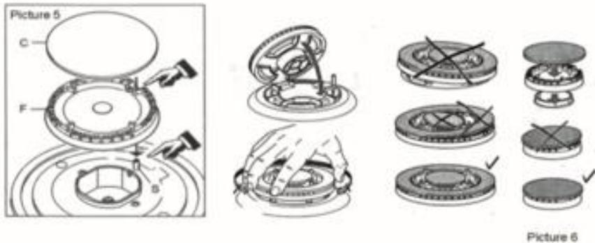
5. Place the burner cap in the correct position after cleaning. Place the flame lid ring in the correct position after cleaning. Refer to picture 6. The burner assembly should not move if installed correctly. Incorrect installation will cause inequality flame quality and may damage appliance.
